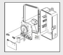
The timer motor is located on the backside of the mechanism and is held in place by a few screws. There are usually 2 wires that go around to the front side to the terminals to provide power to the motor. Remove the wires and motor from the mechanism for replacement.
