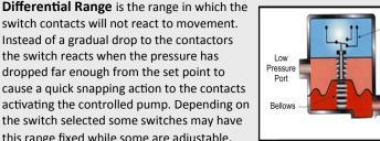
the switch selected some switches may have this range fixed while some are adjustable. **Burst Pressure** is the maximum working pressure the switch can handle before the inner seals and mechanically controlled pieces begin to break apart or fail. Your application should use pressures
