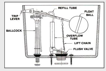
**Refill Tube and Angle Adapter** supply new water to the toilet bowl when the toilet is flushed during the filling process. The refill tube is connected to the overflow tube by the angle adapter. Water is supplied through a barbed fitting on the valve itself.
