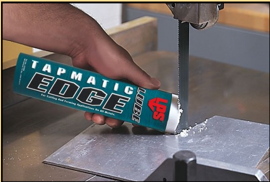
The use of an edge lubricant will help to extend the life of cutting tools and eliminates heat build-up.
